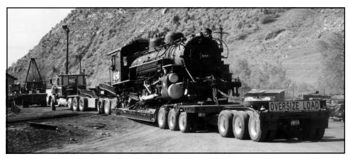
Engine 486 arrives in the D&SNG Durango yard on 5/22/99. The truck was placed over tracks, the trailer under the cab was detached and the trailer dropped to the rails. The locomotive was pulled off the ramp with another locomotive.
